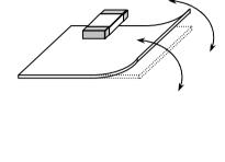
5.2 There is a potential of crack if board is warped due to excessive load by check pin
